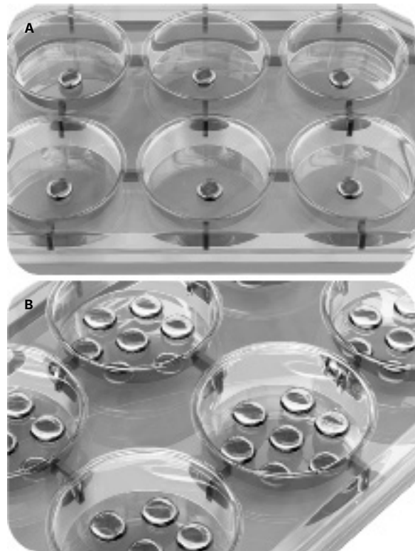
Figure 1. (A) Placement of Cultrex UltiMatrix RGF BME/organoid mixture in the center of a well of a 24-well plate. (B) Placement of multiple domes within a well of a 6-well plate.
