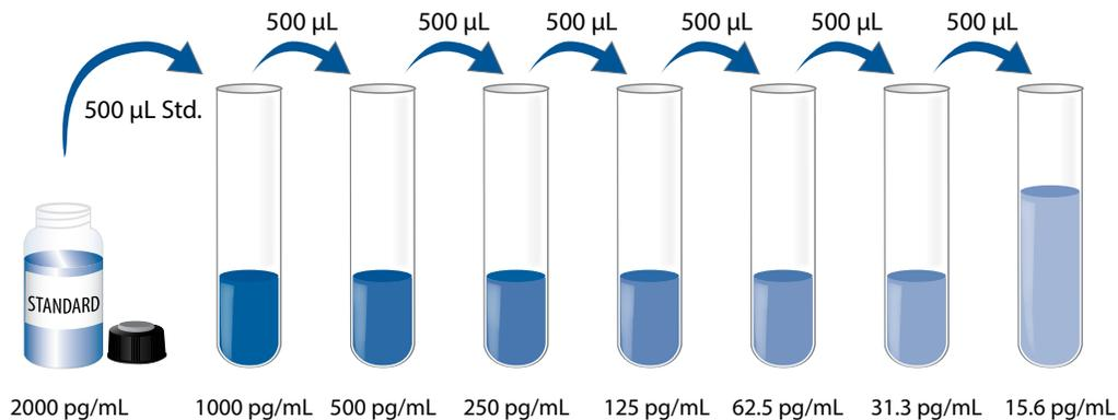
**For Serum/Plasma Samples: Use polypropylene tubes.** Pipette 500  $\mu$ L of Calibrator Diluent RD6U into each tube. Use the stock solution to produce a dilution series (below). Mix each tube thoroughly before the next transfer. The 2000 pg/mL standard serves as the high standard. Calibrator Diluent RD6U serves as the zero standard (0 pg/mL).
