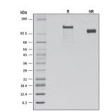
1 µg/lane of Recombinant Human VLDL R (Catalog # 8444-VL) was resolved with SDS-PAGE under reducing (R) and non-reducing (NR) conditions and visualized by silver staining, showing bands at 129 and 107 kDa, respectively.
