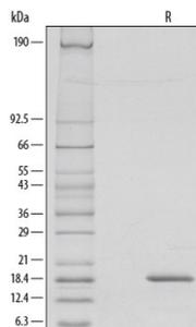
1 µg/lane of Recombinant Human G-CSF was resolved with SDS-PAGE under reducing (R) conditions and visualized by silver staining, showing a single band at 18.5 kDa.
