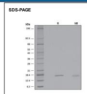
1 µg/lane of Recombinant Human Reg1B (Catalog # 2090-RG) was resolved with SDS-PAGE under reducing (R) and non-reducing (NR) conditions and visualized by silver staining, showing bands at 17.2 and 16.7 kDa, respectively.
