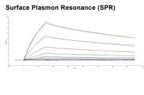
Binding of ACE-2 to SARS-CoV-2 Spike RBD protein with L455F mutation by surface plasmon resonance (SPR). Recombinant SARS-CoV-2 Spike RBD protein L455F His-tag was immobilized on a Biacore Sensor Chip CM5, and binding to recombinant human ACE-2 (Catalog # 933-ZN) was measured at a concentration range between 0.046 nM and 47.2 nM. The double-referenced sensorgram was fit to a 1:1 binding model to determine the binding kinetics and affinity, with an affinity constant of KD= 5.24 nM.
