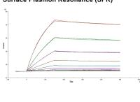
Binding of ACE-2 to SARS-CoV-2 Spike by surface plasmon resonance (SPR). Recombinant SARS-CoV-2 Spike His Protein (Catalog # 10549-CV) was immobilized on a Biacore Sensor Chip CM5, and binding to recombinant human ACE-2 (Catalog # Catalog # 933-ZN) was measured at a concentration range between 0.37 nM and 93.5 nM. The doublereferenced sensorgram was fit to a 1:1 binding model to determine the binding kinetics and affinity, with an affinity constant of KD=1.720 nM. (Biacore T200).
