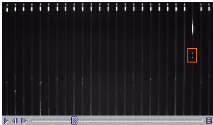
Figure 6-8: Example of a bubble (orange box) in a Wes capillary shown in the fluorescent standard image during the separation movie.
