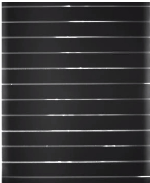
Figure 6-6: Example of fluorescent standards in the separation movie from a plate that was centrifuged with the lid left off. This image was taken after a 60 min separation using a 12 sec stacking load time: 8 sec sample load time. The migration of both the samples and the standards is really variable, and there's significant loss in standard resolution.
